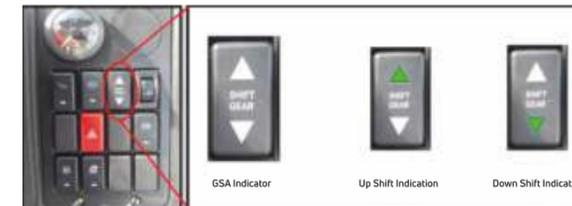
Innovative Gear Shift Advisor for load-terrain based gear shift coaching
