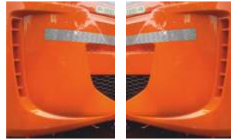
LH & RH aero corners for reduced aerodynamic drag and better fuel economy
