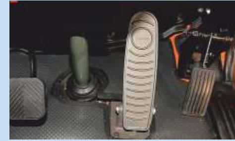
Pendant type accelerator and clutch pedal for fatigueless driving
